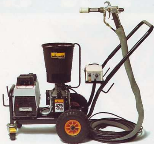
Portable cart system for onsite work consisting of diaphragm airless pump, air compressor, GM2000 Electrostatic Gun, VM200 Power Pack on trolley. Available in both electric diaphragm version or alternatively pneumatic air driven version.
